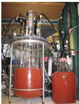
*Membrane bioreactor producing planktonic anammox cells.*
