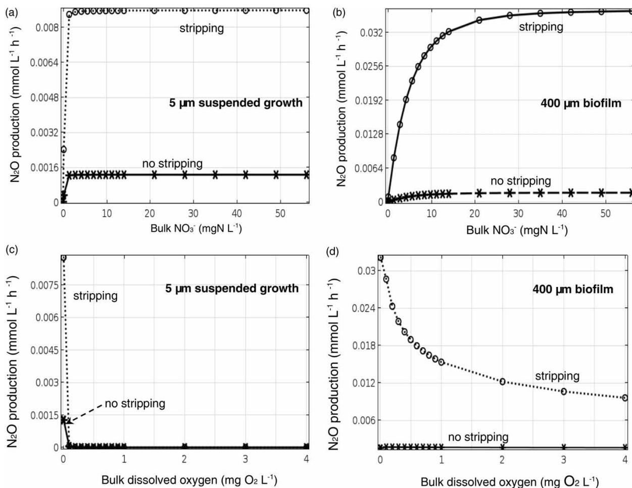
**Figure 5** | N<sub>2</sub>O production rates in denitrifying biofilms with a constant biofilm surface area, with and without stripping, for a 5- $\mu\text{m}$  biofilm ('suspended growth') (a, c) and 400- $\mu\text{m}$  biofilm (c, d) as a function of bulk NO<sub>3</sub><sup>-</sup> (a, b) and (c, d) as a function of bulk O<sub>2</sub>.
