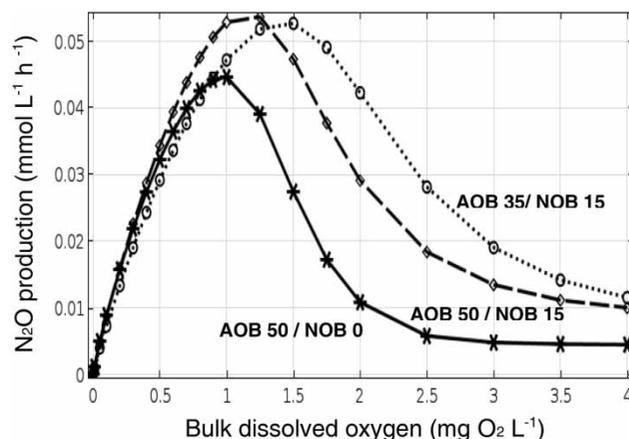
**Figure 2** | Emissions from base case 100 μm nitrifying biofilm with AOB and NOB. The presence of nitrite oxidizers (NOB) in the biofilm may enhance the N<sub>2</sub>O production. N<sub>2</sub>O production rate without NOB (base case, AOB 50 g L<sup>-1</sup>) and with 15 g L<sup>-1</sup> NOB (AOB 50 or 35 g L<sup>-1</sup>).
