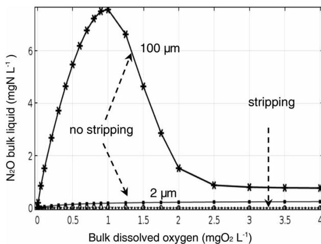
**Figure 3** | N<sub>2</sub>O bulk liquid concentration for nitrifying conditions as a function of bulk O<sub>2</sub> for a 2 μm suspended growth and 100 μm biofilm system, with stripping (solid line) and without stripping (dashed line).
