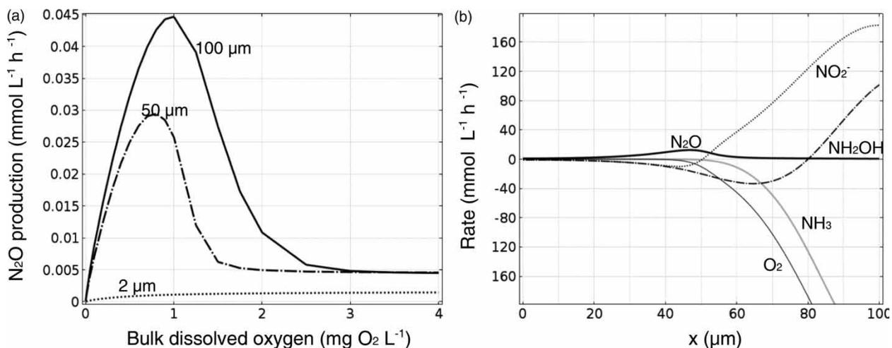
**Figure 1** | (a) N<sub>2</sub>O production rates for AOB biofilms of different thicknesses with a constant biofilm surface area, per unit reactor volume, as a function of bulk O<sub>2</sub>, and (b) net component rates over the biofilm depth (x) for the 100-μm biofilm. Results are for the base case conditions at a bulk O<sub>2</sub> of 0.9 mg L<sup>-1</sup>.
