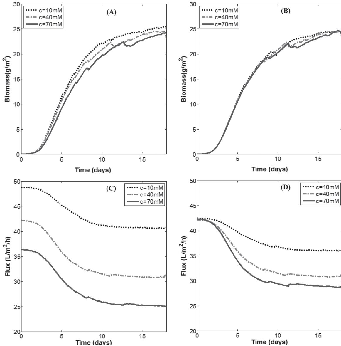
Fig. 3. Compared biomass amount (A, B) and permeate flux (C, D) developed in time at different salt content of the feed (10, 40 and 70 mM). Left: constant operating pressure ( $p = 15$  bar); Right: constant initial flux ( $J = 42$  l/m<sup>2</sup>/h)
