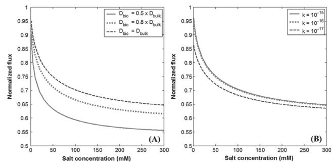
Fig. 6. Influence of (A) effective diffusion coefficient of salt in the biofilm and of (B) biofilm permeability, on the normalized permeate flux (flux in the presence of a 14 d old biofilm related to the flux in the biofilm absence).
