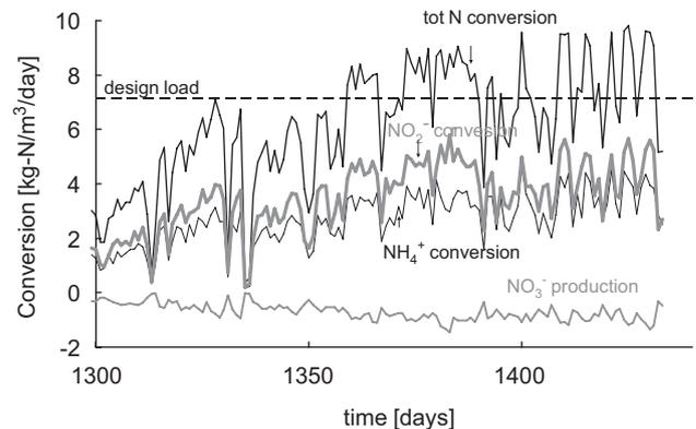
**Fig. 5** – Conversion during the days that the final the design load was achieved. Total nitrogen conversion (thick black), nitrite conversion (thick grey), ammonium conversion (thin black), nitrate production (indicated as negative conversion; thin grey).
