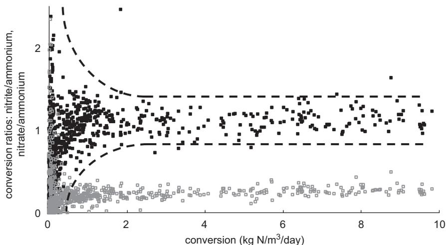
Fig. 7 – Conversion ratio of nitrite and ammonium ( $Y_{NO_2^-/NH_4^+}$  closed squares); ratio between nitrate production and ammonium conversion ( $Y_{NO_3^-/NH_4^+}$  open squares).
