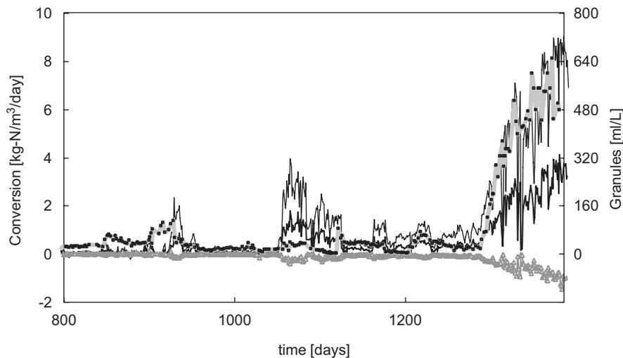
**Fig. 3** – N-conversion rate in the anammox reactor between days 800 and 1400 until the design conversion of  $7.1 \text{ kg-N/m}^3/\text{d}$  was achieved. Conversion of total nitrogen (thin black line), ammonium (thick black line), and nitrate (open triangles, negative, because it is production) are shown on the left axis. The relative volume of granules (thick grey line with black squares, Imhoff value) is shown on the right axis.
