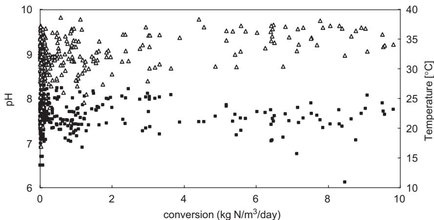
Fig. 8 – pH (closed squares) and temperature (open triangles) at different conversion ratios.
