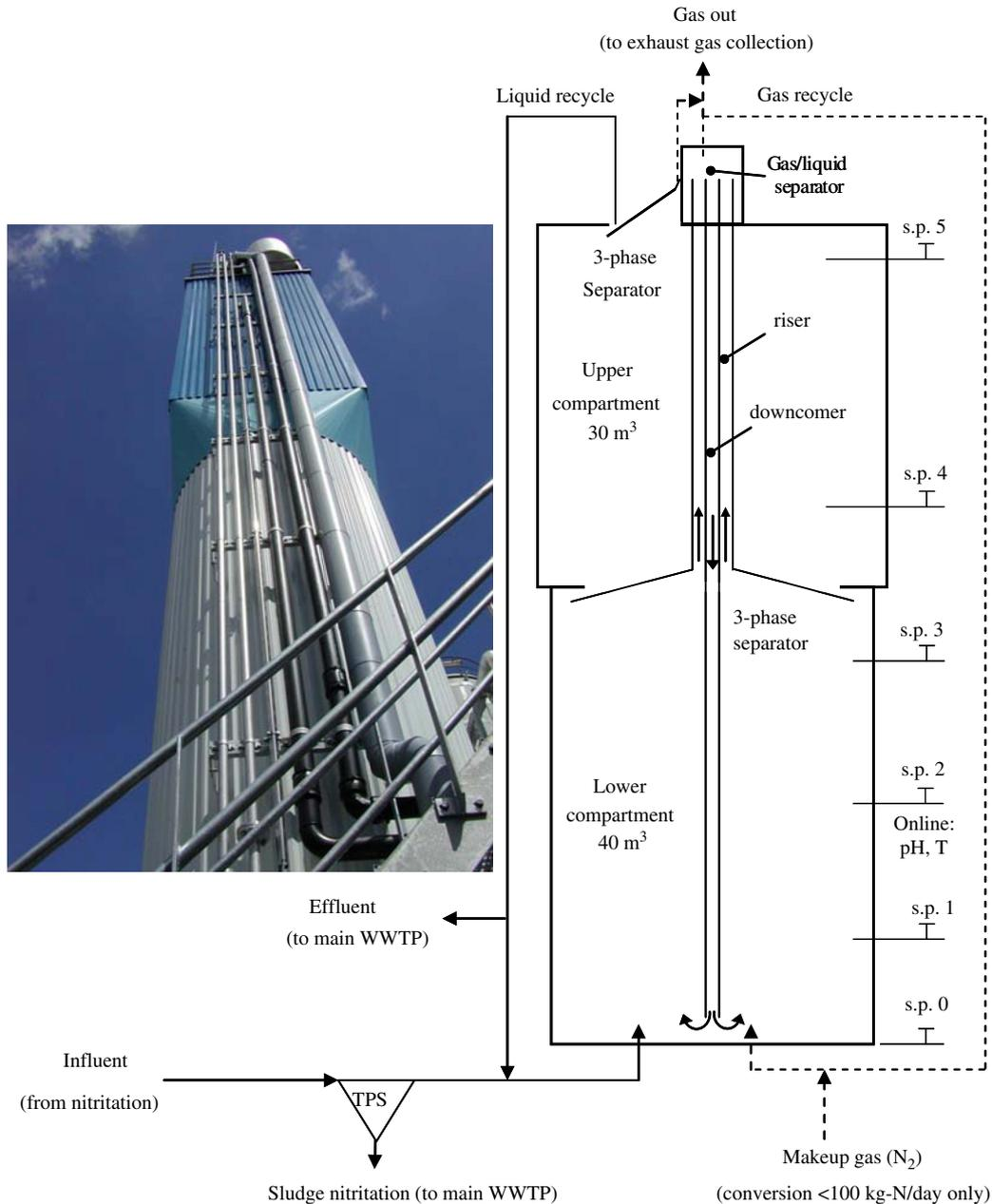
**Fig. 1 – The full (70 m<sup>3</sup>) scale anammox reactor in Rotterdam designed to treat 500 kg-N/d. The photograph shows the upper compartment (dark grey), as well as the lower compartment (light grey). The schematic picture shows the internal gaslift, gas recycle, six sample points (s.p.), as well as the tilted plate settler (TPS) before the anammox reactor.**
