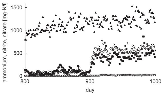
**Fig. 4** – Evolution of concentrations of N-compounds during the transition from operation of SHARON reactor as nitritation–denitrification reactor with methanol addition (until day 900) to operation with nitritation only. Influent ammonium (closed triangles), effluent ammonium (closed squares), nitrite (open diamonds) and nitrate (open circles).
