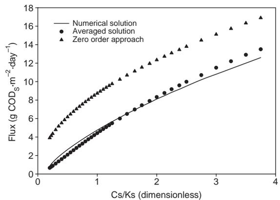
Fig. 4. Direct comparison of numerical, weighted average and zero-order approach in the resolution of Eq. (2). Deviations of both approaches are different from the case of a reactor operating in continuous mode.
