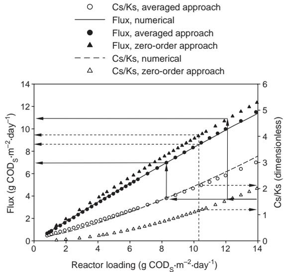
Fig. 3. Comparison between numerical and weighted average and zero-order approach for a steady-state biofilm in a wide range of inflow concentrations in a well-mixed tank operating in continuous mode. Arrows show differences when using the half-order approach for a fixed  $C_S/K_S$  (designing a biofilm reactor, solid arrows), and for a fixed reactor loading (describing existing reactor systems, dashed arrows).
