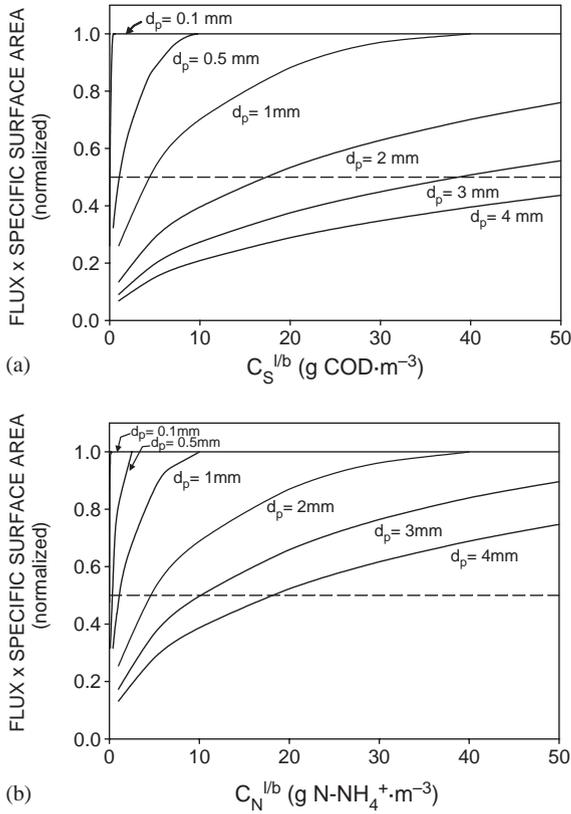
Fig. 6. Effect of particle diameter ( $d_p$ ) in the flux times specific surface area in a granular or flocculated sludge: (a) heterotrophic system; (b) autotrophic  $NH_4^+$  oxidizing system.
