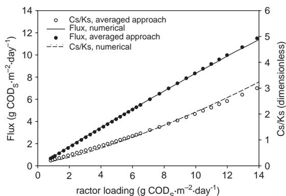
Fig. 1. Comparison between numerical and weighted average approach for a steady-state biofilm in a wide range of inflow concentrations in a well-mixed tank operating in continuous mode.
