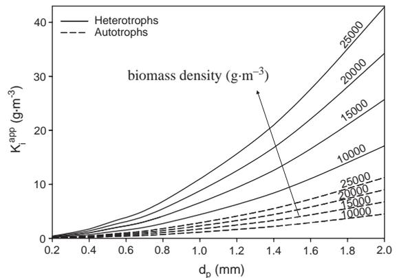
Fig. 7. Effect of floc diameter ( $d_p$ ) and biomass density on the apparent affinity constant for heterotrophs and autotrophs in a flocculated activated sludge system.
