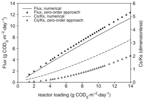
Fig. 2. Comparison between numerical and zero-order approach for a steady-state biofilm in a wide range of inflow concentrations in a well-mixed tank operating in continuous mode.
