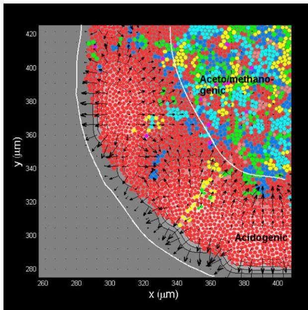
**Figure 5** Hydrogen flux (arrows) in a small (200  $\mu\text{m}$  upper limit) granule, fed mostly sucrose (Subscribers to the online version of *Water Science and Technology* can access the colour version of this figure from <http://www.iwaponline.com/wst>.)
