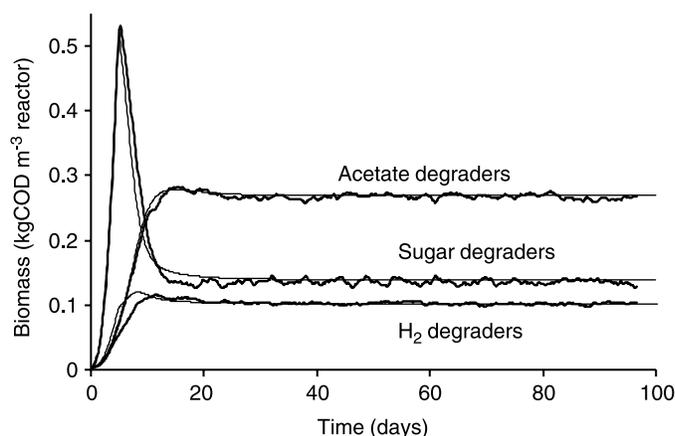
**Figure 2** Evolution over time of different biomass types in the Aquasim 2.1d biofilm model (thin line), and multidimensional model (heavy line) for a planar biofilm with upper size limit of  $140 \mu\text{m}$
