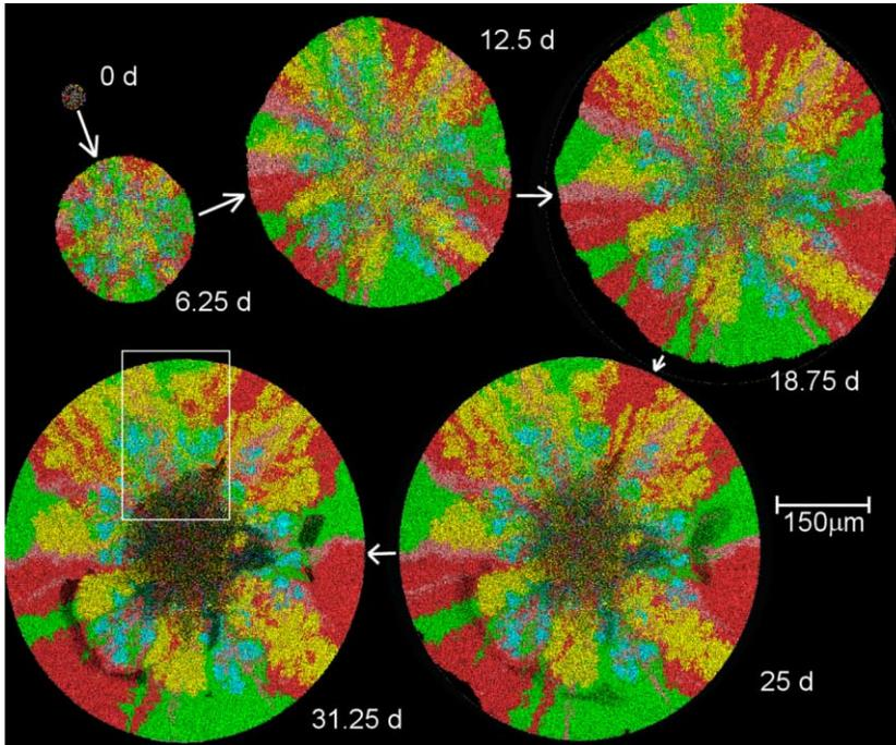
**Figure 3** Growth of a granule (600  $\mu\text{m}$  upper diameter) over 31 days on mostly organic acid feed, with different microbial types in different shades. The area in the centre after 25 days is mostly unoccupied due to biomass decay. The highlighted region at 31.25 days refers to Figure 4 (Subscribers to the online version of *Water Science and Technology* can access the colour version of this figure from <http://www.iwaponline.com/wst>.)
