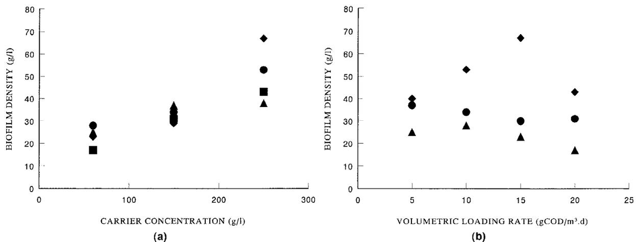
**Figure 4.** Influence of carrier concentration (A) and volumetric substrate loading rate (B) on biofilm density expressed as gram of biomass per L of biofilm volume (excluding pores). Symbols: A: (▲) 5, (●) 10, (◆) 15, (■) 20 kgCOD/m<sup>3</sup> · d; B: (▲) 60, (●) 150, (◆) 250 g-carrier/L.
