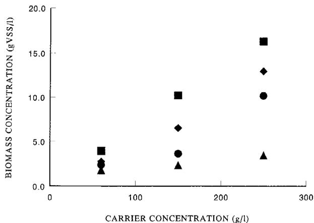
**Figure 5.** Biomass concentration as a function of basalt concentration and loading rate; loading rate: (▲) 5, (●) 10, (◆) 15, (■) 20 kgCOD/m<sup>3</sup> · d.
