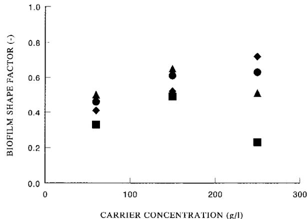
**Figure 6.** Observed effect of the carrier concentration and volumetric loading rate on the shape factor of the biofilm particles (Shape factor 1: fully circular biofilm). Loading rate: (▲) 5, (●) 10, (◆) 15, (■) 20 kg COD/m<sup>3</sup> · d.
