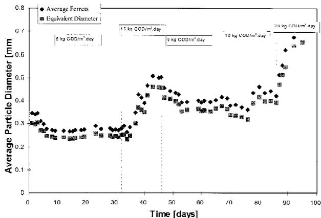
**Figure 2.** Average biofilm particle diameter vs. time in a BAS reactor with  $150 \text{ g}_{\text{basalt}}/\text{L}$  (Experiment E2, see Table I). Average diameter of basalt carrier: 0.2 mm.
