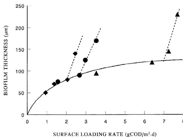
**Figure 7.** Effect of substrate surface loading rate and carrier concentration on biofilm thickness. Carrier concentration: (▲) 60, (●) 150, (◆) 250, kg/m<sup>3</sup>.
