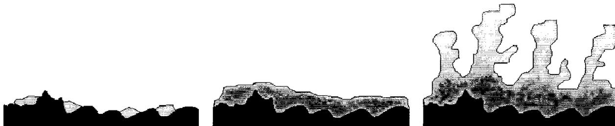
**Figure 1.** Schematic representation of the postulated influence of substrate surface loading rate (increases from left to right) and detachment force (decreases from left to right) on biofilm structure (adapted from Van Loosdrecht et al., 1995b).
