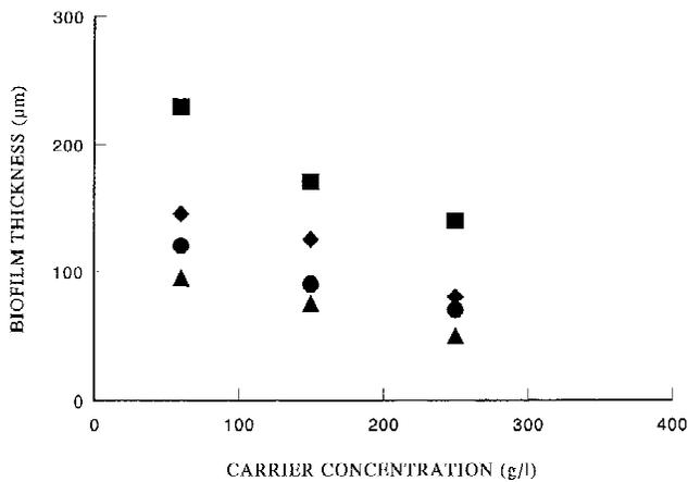
**Figure 3.** Relation between biofilm thickness and carrier concentration at different substrate loading rates. Loading rates: (▲) 5, (●) 10, (◆) 15, (■) 20 kg COD/m<sup>3</sup> · d.
