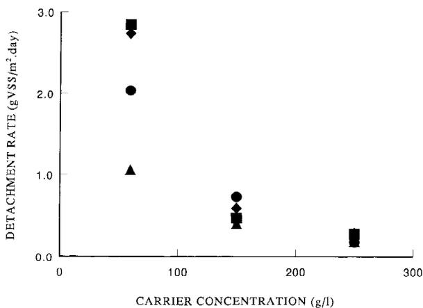
**Figure 11.** Biomass detachment force at different carrier concentration. Loading rate: (▲) 5, (●) 10, (◆) 15, (■) 20 kg COD/m<sup>3</sup> · d.
