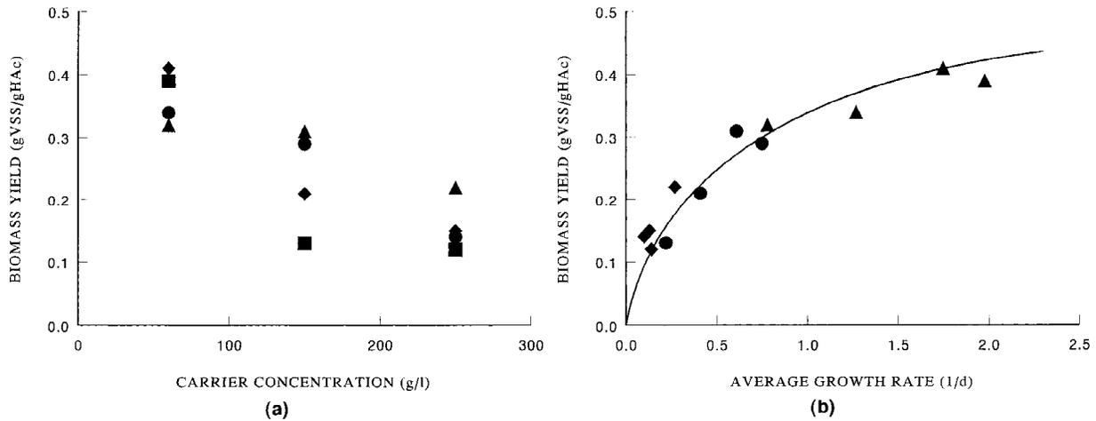
**Figure 10.** Observed biomass yield as a function of carrier concentration (A) and average specific growth rate (B). (A) Loading rate: (▲) 5, (●) 10, (◆) 15, (■) 20 kg COD/m<sup>3</sup> · d; (B) Carrier concentration: (▲) 60, (●) 150, (◆) 250, kg/m<sup>3</sup>.
